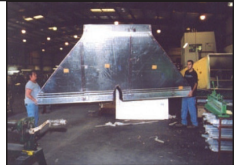
Certified KoolDuct fabricators Malinda Bostic and Nick Dean easily move a huge unit tie-in.
