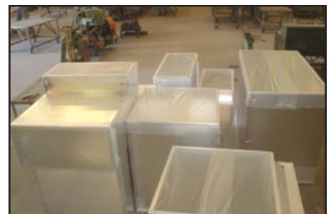
McDonalds protected storage maintains contaminant free ductwork interior. In this photo the ends have been sealed for shipment.
